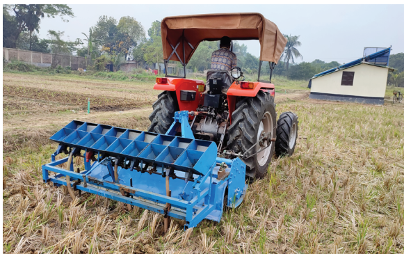
Fig. 2. Pictorial view of strip tillage by four-wheel operated seeder
